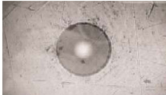
Figure A.3* Scratched connectors must be rejected.
