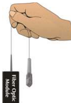
Figure A.1 Improper handling of a pigtailed device.
