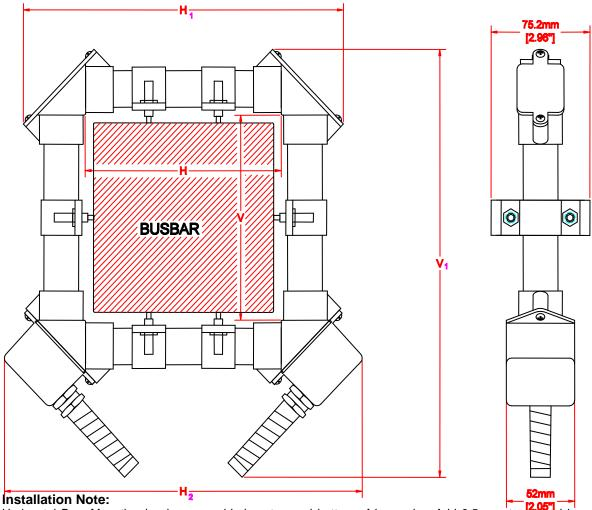
Horizontal Bus: Mounting hardware provided on top and bottom of bus only. Add 3.5 mm to vertical bus dimension to accommodate mounting hardware.
