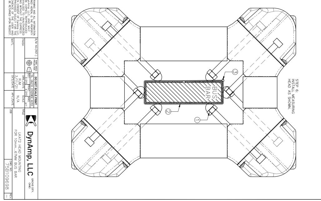
NOTE: 1.) IF ONE ZIP TIE IS NOT LONG ENOUGH TO ENCIRCLE BUS BAR AND BUCKLE, USE TWO ZIP TIES BUCKLED TOGETHER. POSITION THE BUCKLE(S) AT CORNER(S) OF BUS BAR.
