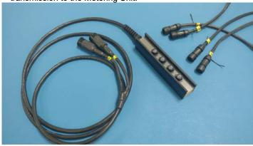
The Metering Unit is powered by 18...36V from the included universal power adapter or an external DC supply. Even battery.
